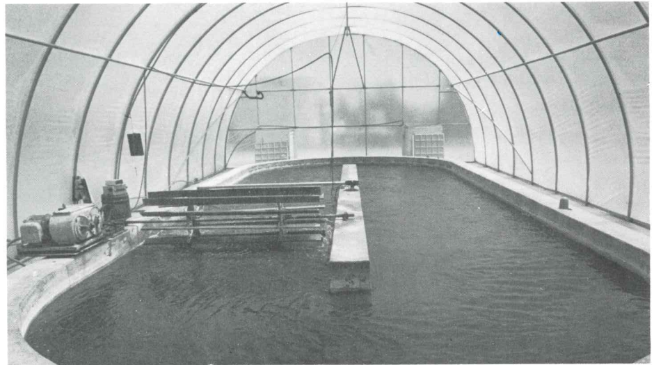
This greenhouse raceway is one of five algae ponds at the Roswell Test Facility that will be used to test algae production methods.
